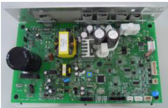
LCB without the transfer board (Part number # 1000203336 )
